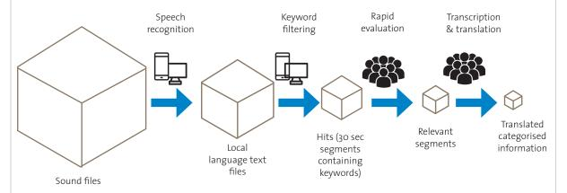
Overall radio mining process for converting a large quantity of unstructured audio data into a small quantity of relevant, structured information. ©UN Global Pulse, 2017
